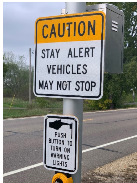
Unique signage at an RRFB crossing designed in partnership by SRF and Dakota County.
