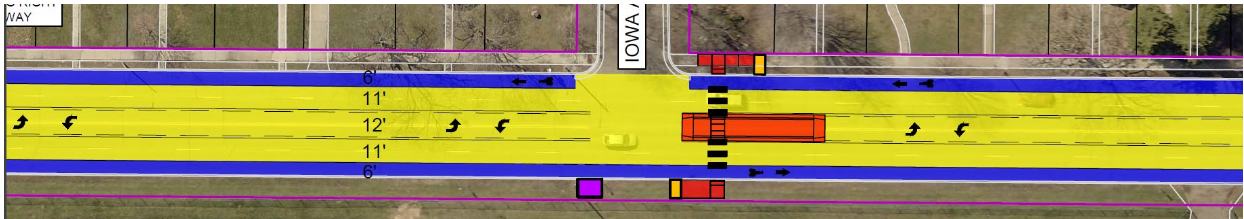
Proposed Three-lane (top) and Exemplar Pedestrian Refuge (bottom)
