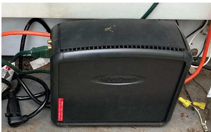
Uninterruptable Power Supply (UPS)
